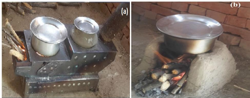
**Fig. 3** Types of chulha in rural India: **a** improved metal chulha (IMC) and **b** traditional mud chulha (TMC)
